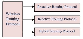
Figure1: Types of Wireless Routing Protocol
